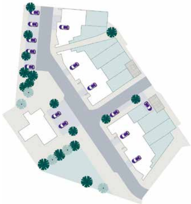
Figure 129 Well considered on street parking interspersed with landscaping and bin storage areas
