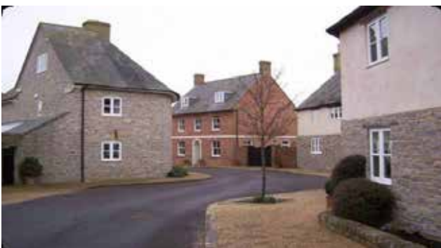
Sharp bends and restricted forward visibility used as a speed control measure. Image courtesy of Andy Cameron.
