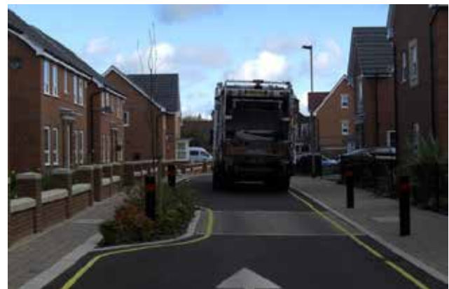
This small housing development has a simple U-shaped one-way system street layout and controlled on-street parking in place, which aids refuse collection vehicles in navigating the site.
