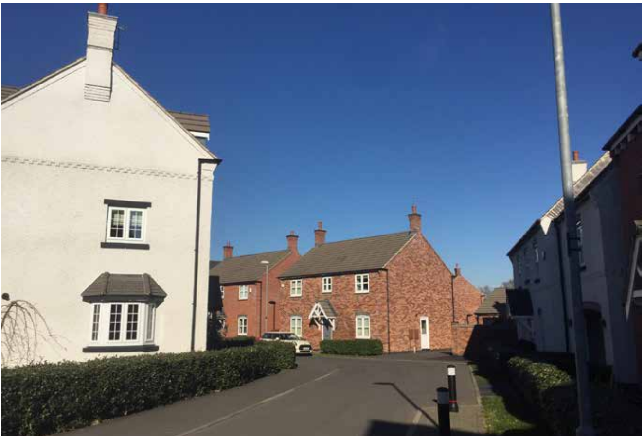
Figure 125 Reduced forward visibility on street in Lount, Leicester helps to reduce vehicle speeds
