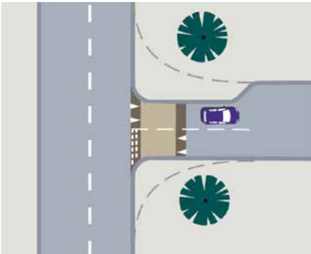
Figure 126 Continuous footways should be used
